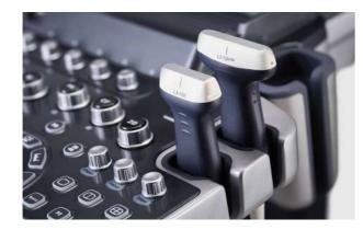
The high-density linear transducers can be attached to the E-CUBE 8 LE. Several footprint width options and high-quality linear images help with breast/thyroid/musculoskeletal/vascular examinations
