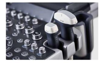
PowerView<sup>™</sup> technology is applied to the Convex and Phased array transducers. PowerView™ technology disperses heat generated by the transducers, improving its durability and ensuring the stability of diagnosis. The increased efficiency of ultrasonic waves enhances signal sensitivity and improves the clarity of clinical images.
